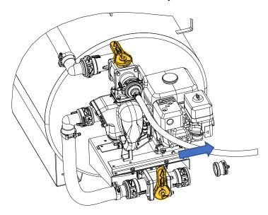
2. Turn the outlet valve handle to the right to empty the sealer from the tank.
