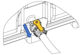
5. Start the engine and pump the sealer from the tote to the tank.
