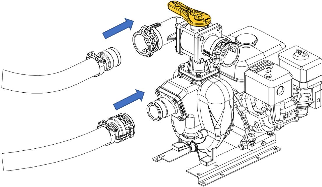
4. Connect the 2" male camlock connection from the spray wand assembly to the other side of the pump valve
