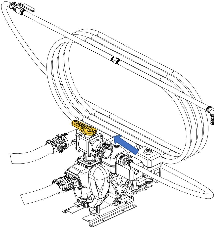
5. Open the valve on the tote outlet before beginning operation
