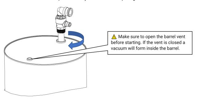
2. Connect the 2" and ¾" female camlocks to the appropriate connections on the barrel adapter.
