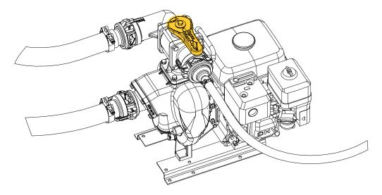
**3.2 Spray Wand Operation**The spray wand included with this system has a ball valve handle to accurately control the flow of sealer. Please refer to the following diagram for the valve positions.
