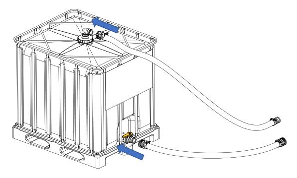
3. Connect the 2" male camlock connection to the pump valve and the 2" female camlock connection to the pump intake.
