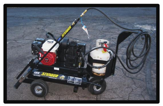
The Stinger is a portable heat lance on wheels. The unit is a one person operation, ideal for the medium to small pavement maintenance contractor who needs a quality heat lance but does not have access to a large tow behind compressor. The Stinger comes complete with electronic ignition and stainless steel burner and regulator. A 25 foot hose kit makes for easy access to cracks or the lance can be maneuvered with the lance in its holder as shown.
