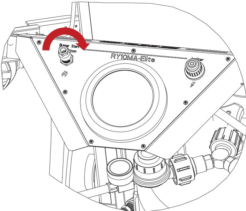
Simply thread the cap with your fingers over the button on the flame-out valve until snug.
