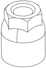
The cap is designed to screw onto the top of the flame-out valve.
