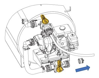
2. Turn the outlet valve handle to the right to empty the sealer from the tank.
