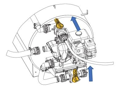
5. Start the engine and pump the sealer from the drum to the tank.
