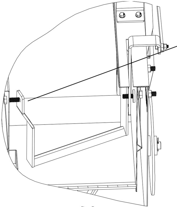
Attach the agitation sweep bar by reassembling the bolts to the agitation connector handle
