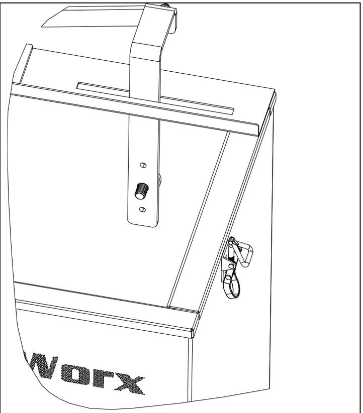
Remove the nut threaded on the stud and install the agitation sweep bar as shown, put it over the left stud first and then the right
