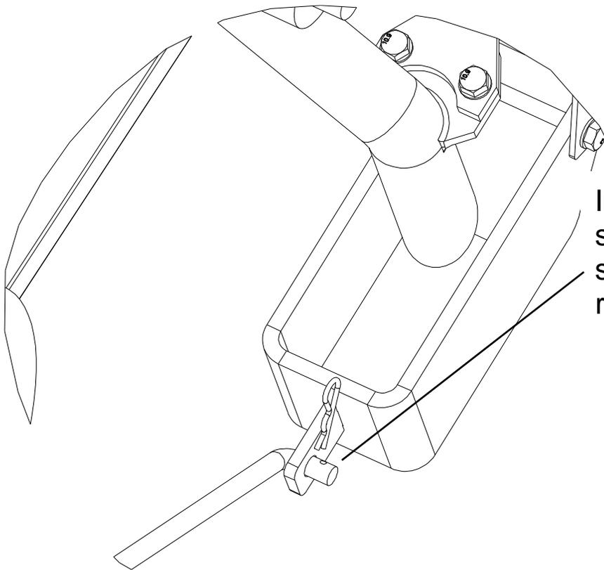
Insert the lower end of the shoe control rod into the shoe tab and insert the retaining pin.
