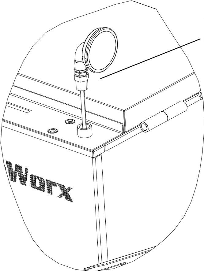
Thread the thermometer into the kettle
