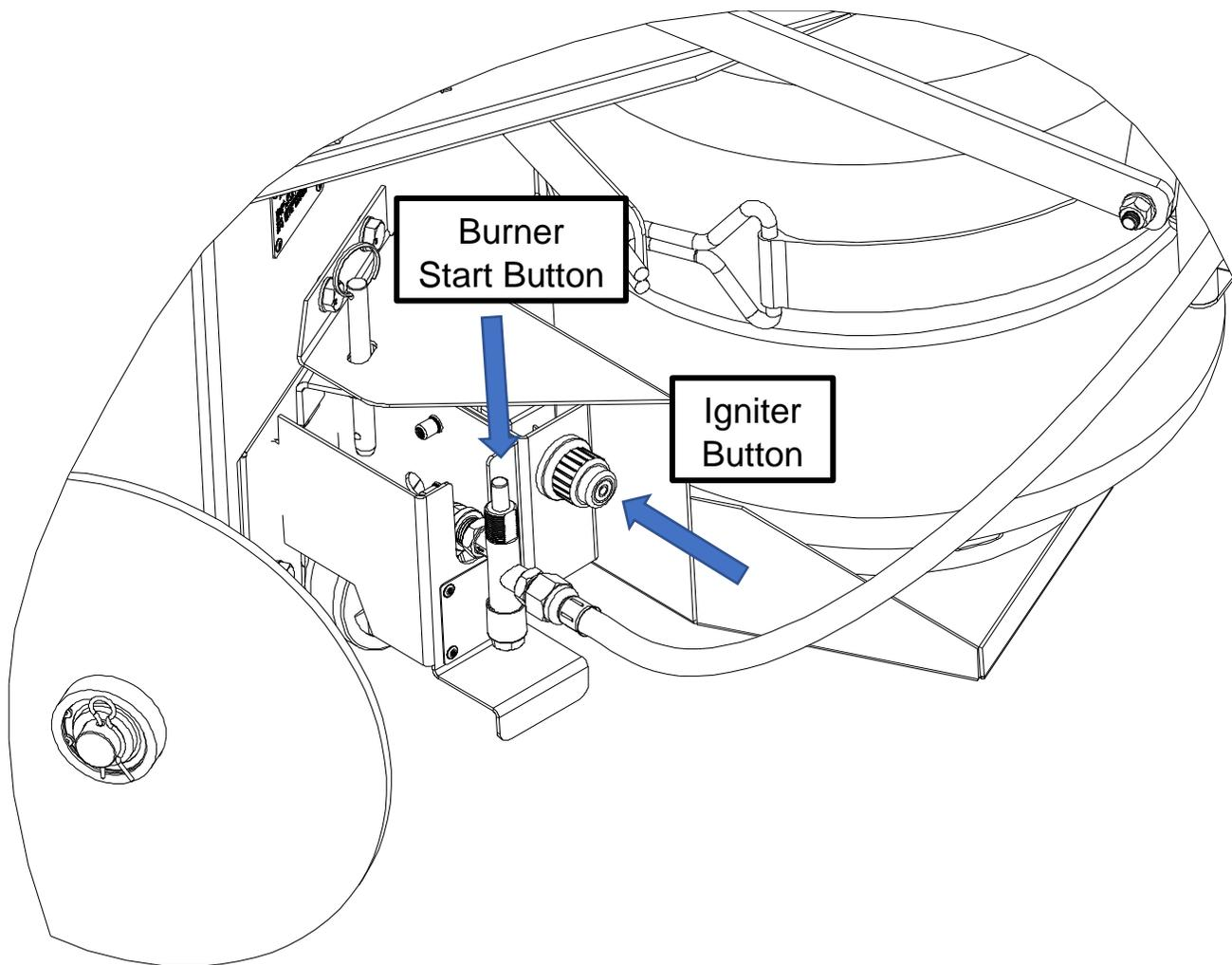
⚠ Operating the burner on high in most conditions is not recommended, this can harm sensitive electronic components and dangerously overheat fuel carrying lines.
