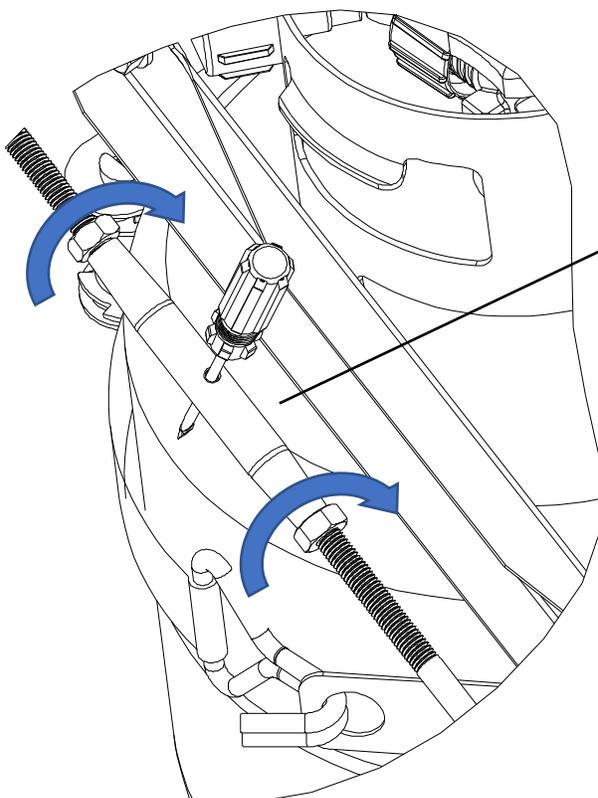
Once the control rod lengths are set, use a screwdriver to hold the turnbuckle in place and tighten the nuts against the turnbuckle
