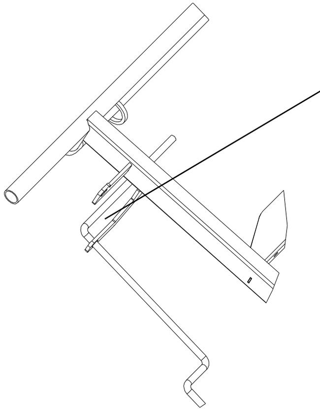
Insert the shoe control handle into the lower guide
