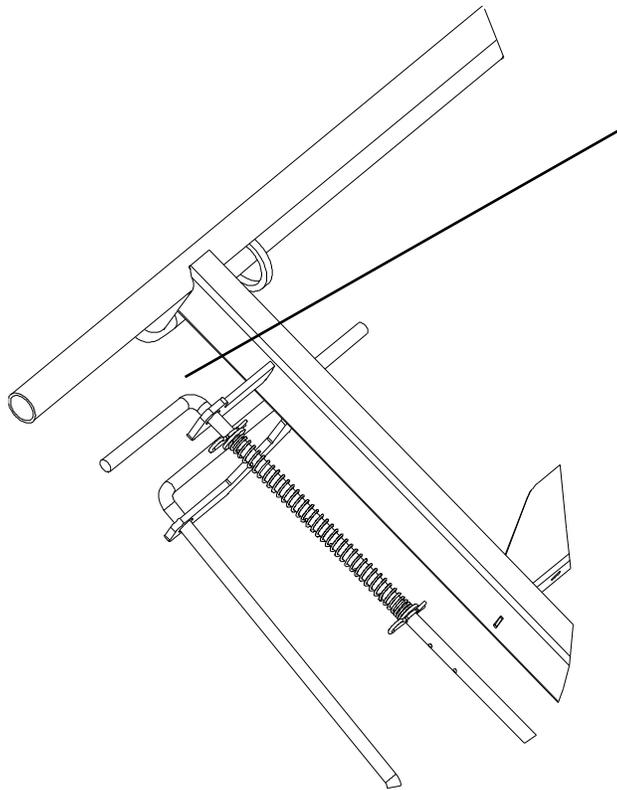
Insert the valve control handle into the upper guide
