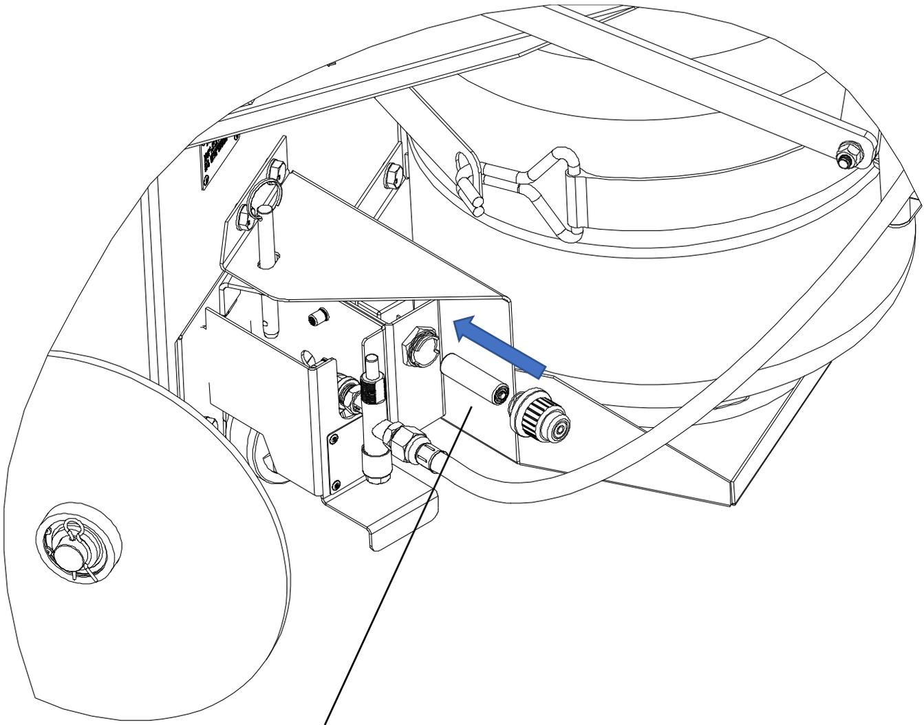
Unthread the igniter cap and insert the AA battery with the positive terminal facing up
