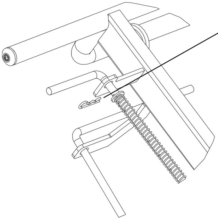
Remove the spring retainer pin to put tension on the valve control rod
