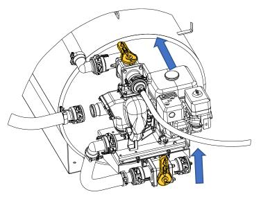
5. Start the engine and pump the sealer from the drum to the tank.
