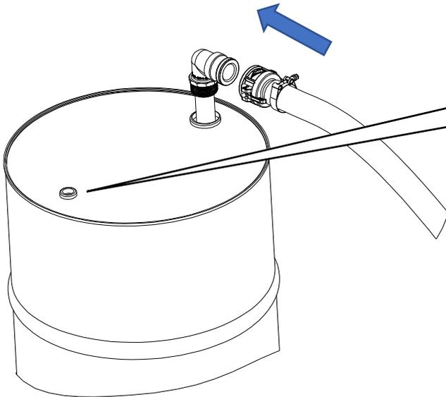
⚠ Make sure to open the barrel vent before starting. If the vent is closed a vacuum will form inside the barrel.
