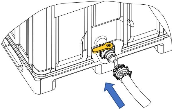
2. Disconnect the female camlock on the pump intake (ensure that the tank outlet valve is closed by making sure the valve handle is in the upright position).
